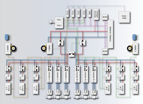
**Engines:** Only two of the six electric propellers are needed for the stable, long-lasting Antares E2 flight in the event of a crisis.
